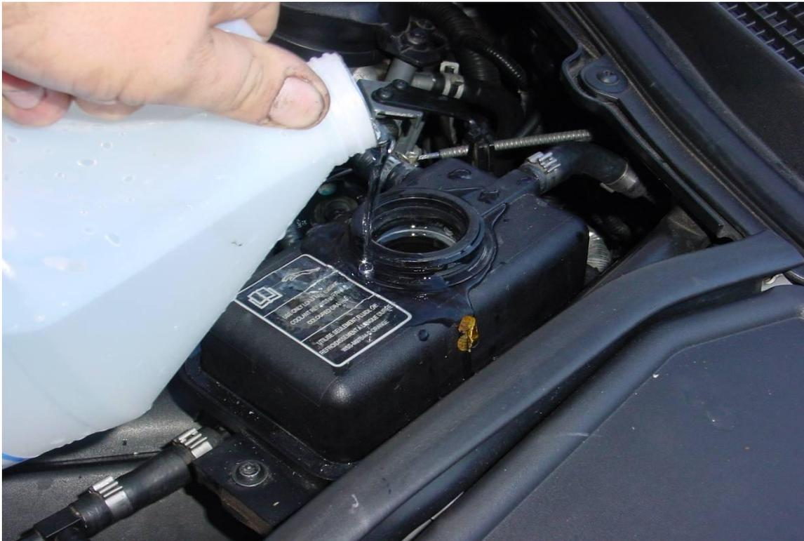
**\*\*\*Step 10)** ...and add clean tap water to intercooler plug until drain runs clear.
