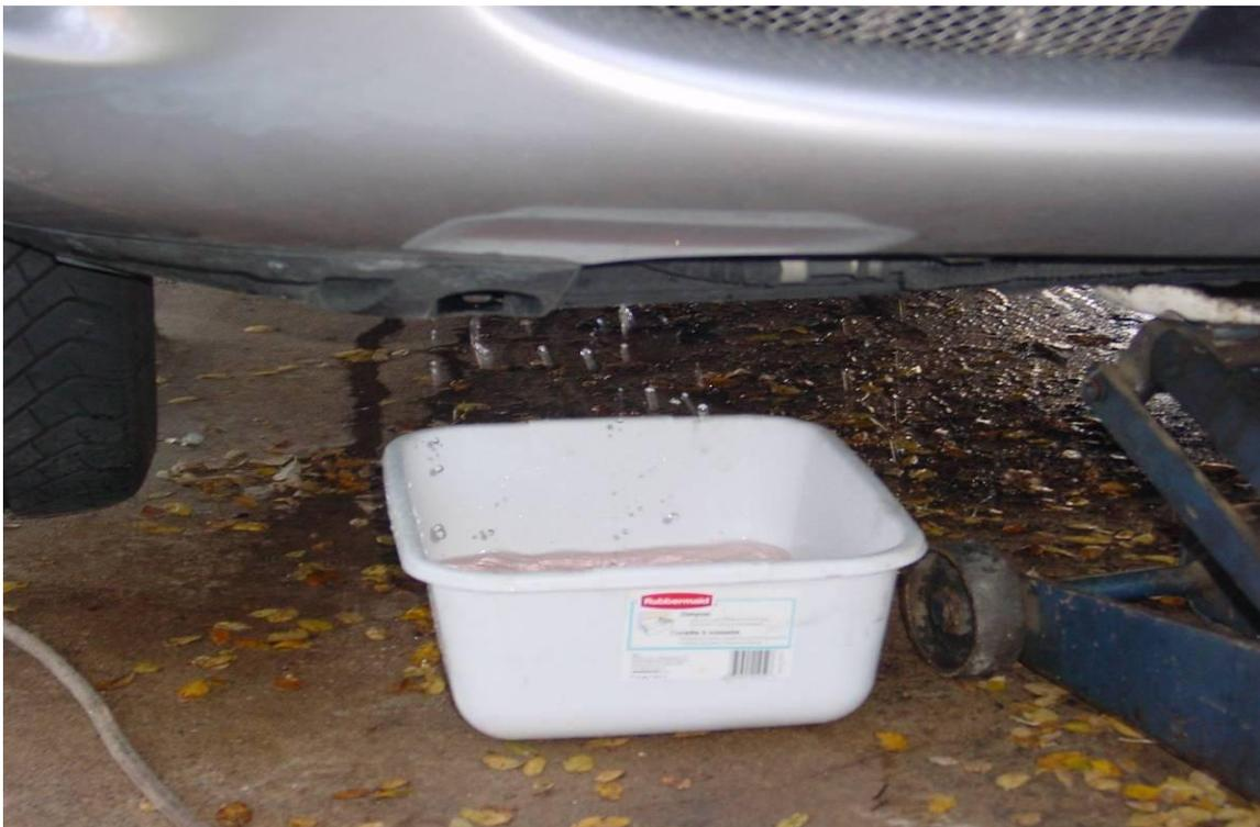
**Step 6)** Remove jackstands and lower car to the ground to assist draining.
