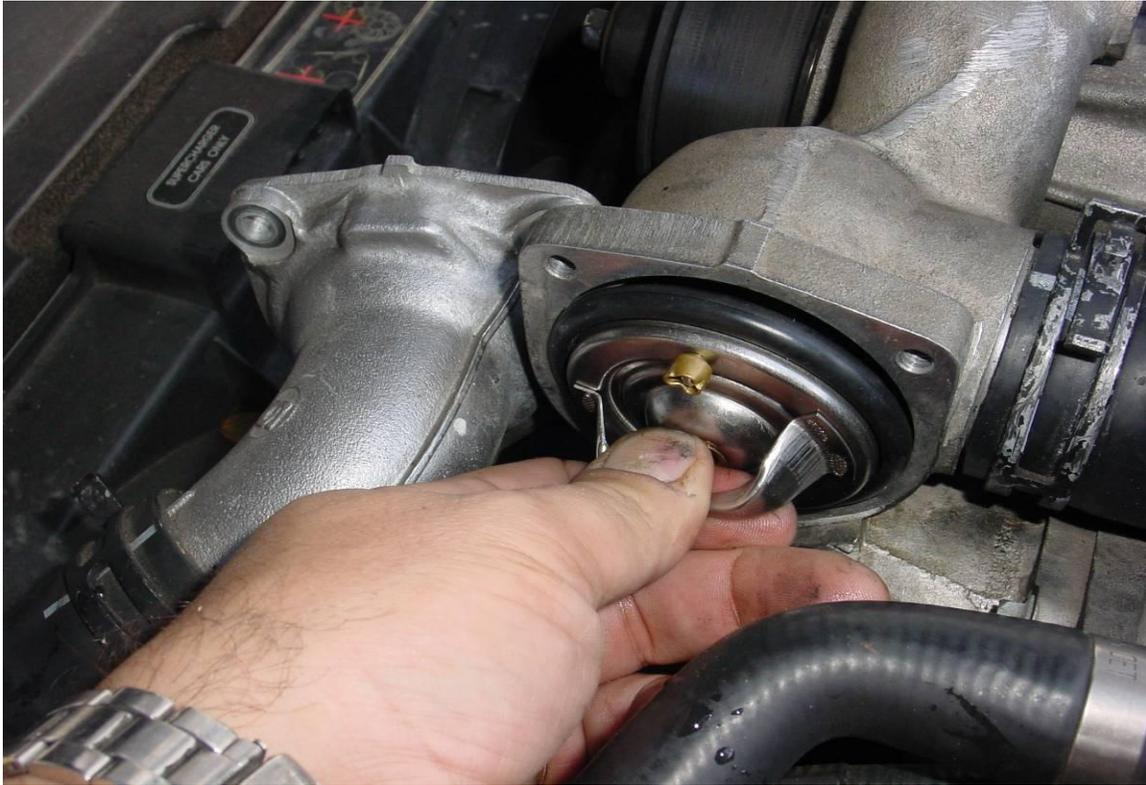
**Step 25)** Install cover and torque bolts to 8-10 Nm (6-7.4 ft-lbs).
