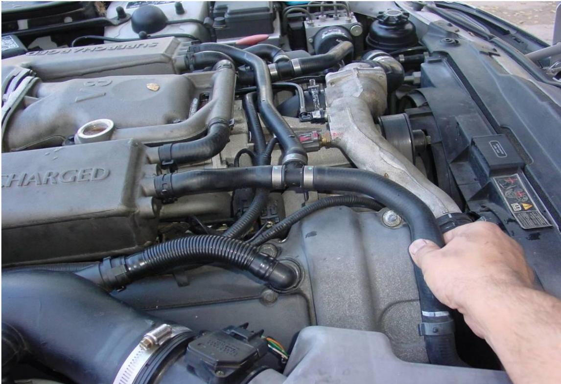
**\*\*\*Step 17)** Using the tool made in Step 1, install intercooler coolant plug.
