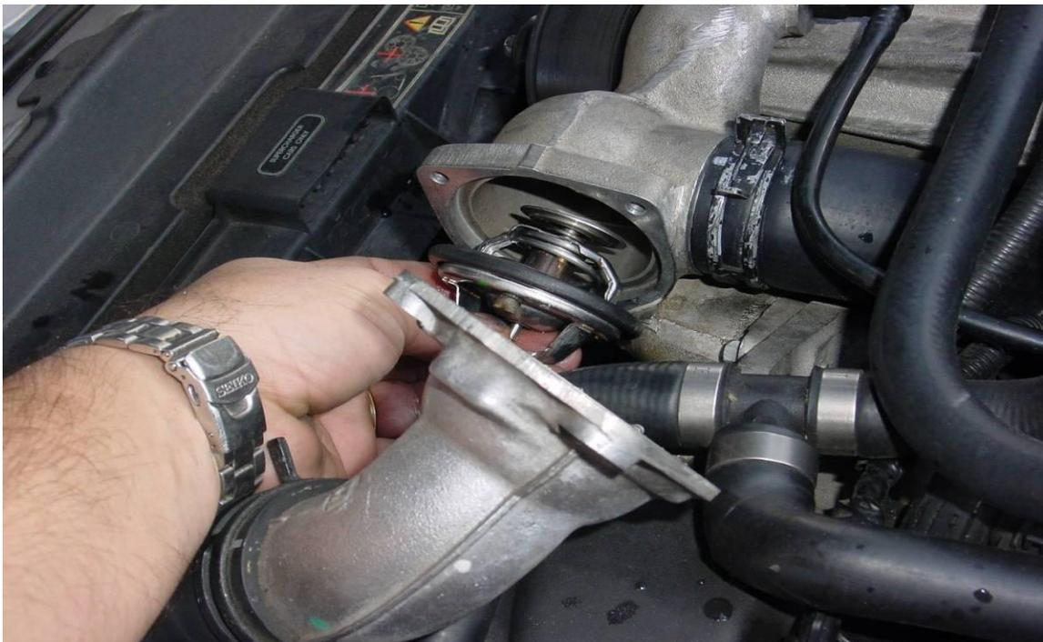
**Step 24)** Install the new thermostat with the air bleed valve (brass with ball bearing) at the top, as shown.
