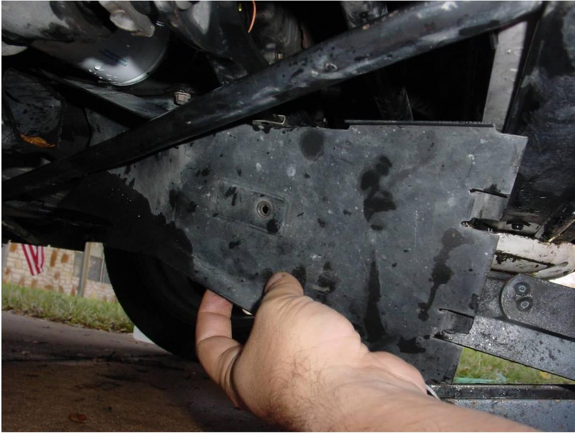
... and with the duct removed, we can now see the radiator drain plug (at right in the picture). This is on the right-hand end of the radiator on the engine side.
