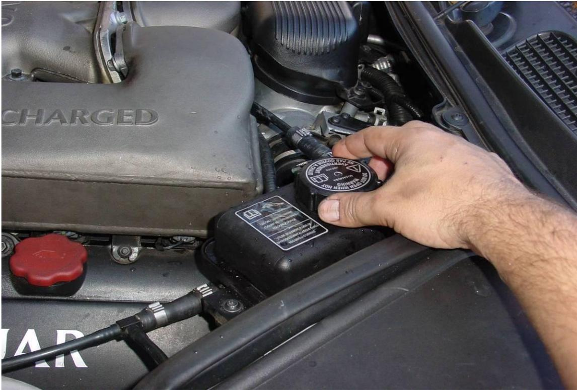
**\*\*\*Step 16)** Fill the system at the intercooler plug. You can “burp” air out of the system when the water level nears the top by squeezing the intercooler hose as shown.
