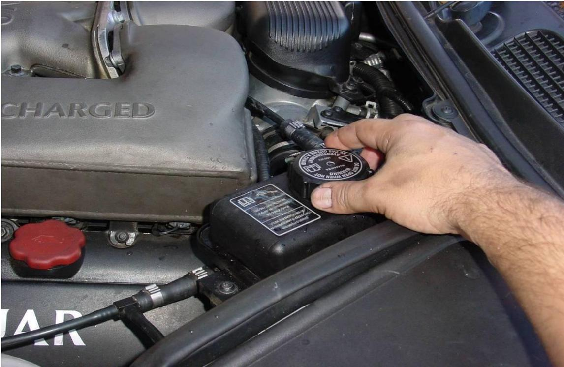
**\*\*\*Step 8)** Using the tool made in Step 1, remove the intercooler coolant plug.
